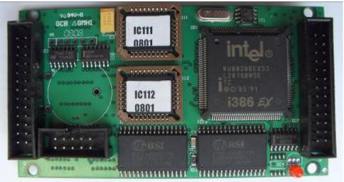
C. Remove IC111 and IC112 as shown in the figure.
