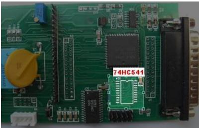
G. Install IC111 and IC112. Make sure the install direction is correct. See the figure.
